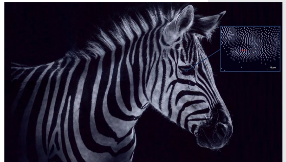
Selective laser ablation on a sapphire substrate removing a 10 nm thickness ceramics layer
