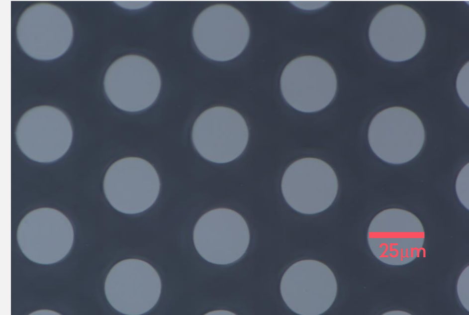
No chipping or micro cracks
