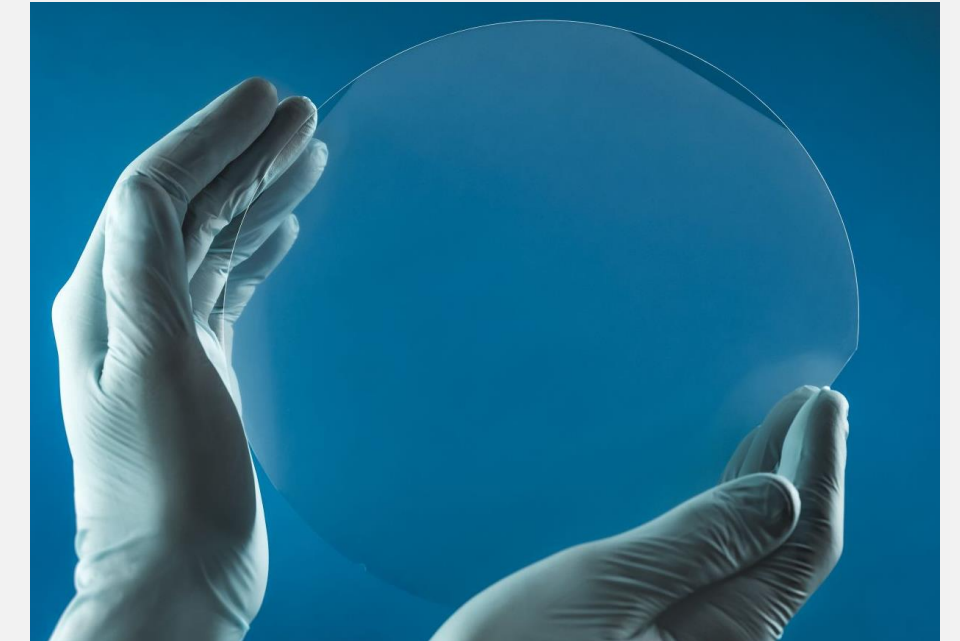
HIGH SPEED: 45 min., takt time. 3 M holes in 200 mm diameter and 500 \mu\text{m} thickness fused silica wafer.
