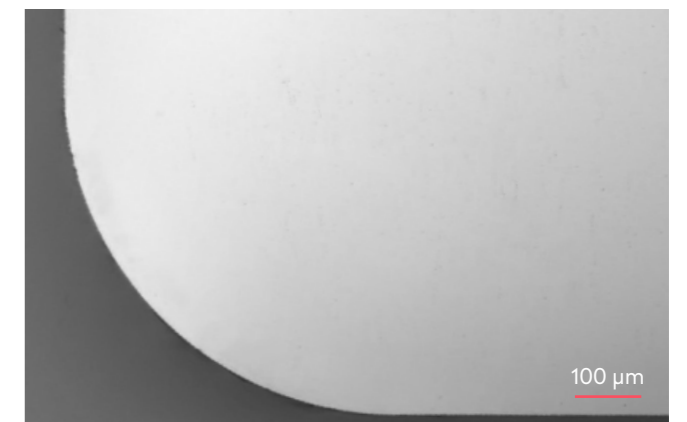
Sapphire laser cutting, thickness 600 µm
