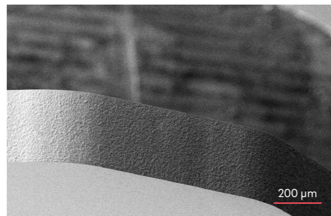
D236T glass laser cutting, thickness 300 µm
