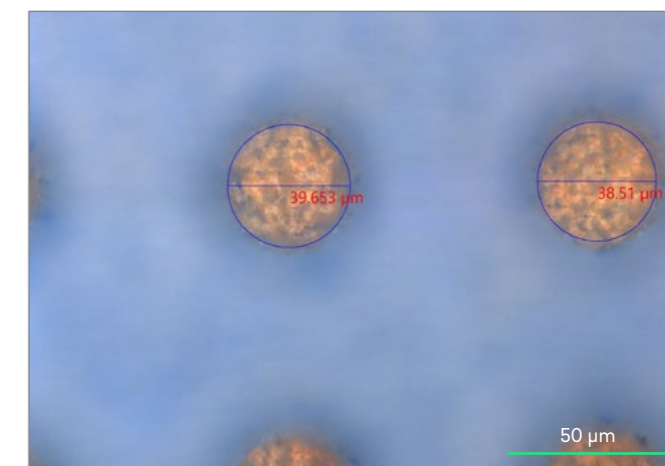
Blind holes drilling in multi layered sandwich like substrate - 25 \mu\text{m} thickness dielectric layer (blue color) drilling to gold layer (yellow color).
