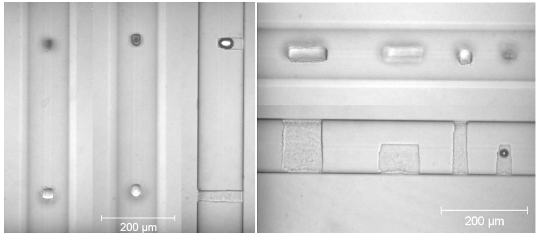
Fig. 2 Rectangular holes (through and blind) drilled in 125 μm diameter single mode fibers for fiber Fabry-Perot interferometer (FFPI) applications: measurement of refractive index of material filling the hole, temperature, deformation, flow, etc.
