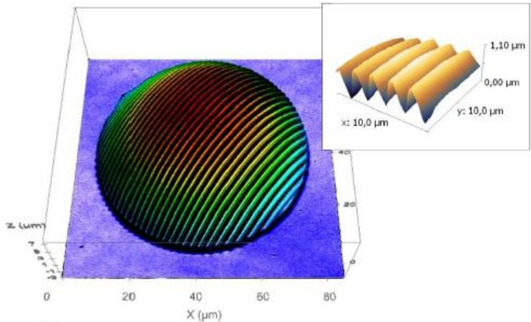
Fig. 4: Hybrid micro-lens with a phase grating, allowing different light flow control variants to be achieved. The grating gives diffraction which can be used as a light dispersing element or as a spectral filter. The grating itself can have not only geometry of parallel lines, but also of perpendicular lines or concentric rings, for ex. lenses with Fresnel zones. The curvature radius of the lens is  $R = 67 \mu\text{m}$ , grating period  $d = 2,4 \mu\text{m}$ .
