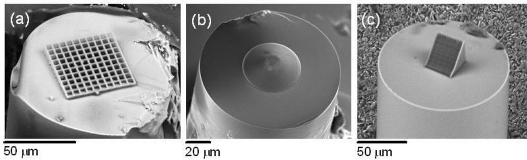
Fig.2 Microoptics on fiber-top
