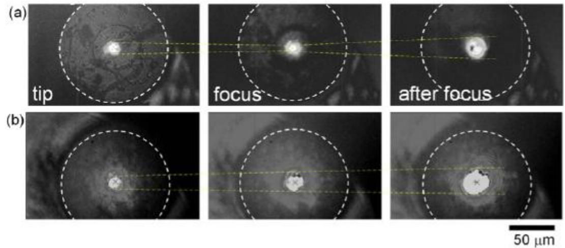
Fig. 3: Focusing of light emitted from the fiber with the tip-lens (a) and without (b). The dashed-circle marks the circumference of the fiber tip; lines are eye guides for the focusing and diffraction. The focus of imaging plane is at the fiber tip  $z = 0 \mu\text{m}$  (left), at the focus  $z = 33 \mu\text{m}$ , and  $z = 100 \mu\text{m}$  from the tip of fiber (right side images).
