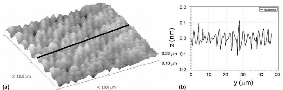
Fig. 5: Surface roughness of a fs-laser polymerized SZ2080 lenses is below ~30 nm. (a) shows typical AFM measured profile and (b) line-marked cross section.
