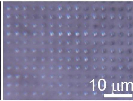
2. Front and back illumination optical micrograph of perforated foil, back surface.
