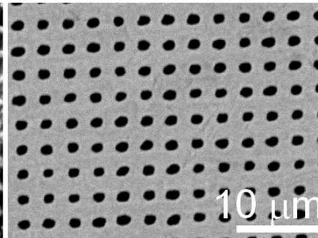
4. SEM micrograph of perforated foil, back surface.
