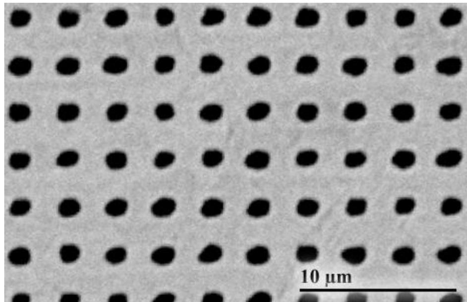
Fig. 1 Precise micro holes drilling (down to 1  $\mu\text{m}$  diameter).
