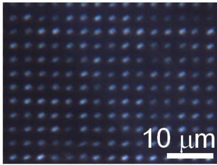
1. Front and back illumination optical micrograph of perforated foil, front surface.
