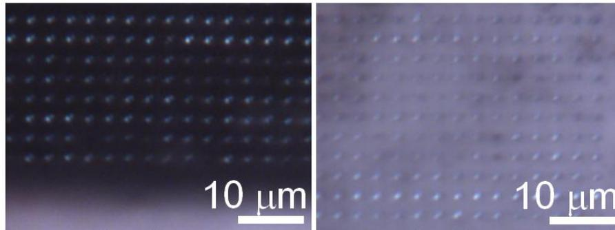
1. Front and back illumination optical micrograph of perforated foil, front surface.
