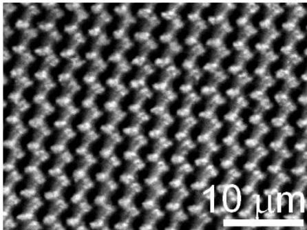
3. SEM micrograph of perforated foil, front surface.
